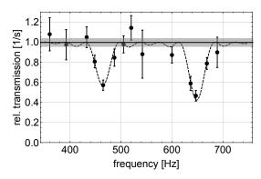
**Figure 9** Taux de transmission des neutrons en fonction de la fréquence. Figure extraite de G. Cronenberg et al., A Gravity of Earth measurement with a qBounce experiment, Proceedings of the EPS Conference on High Energy Physics 2015, arXiv:1512.09134
